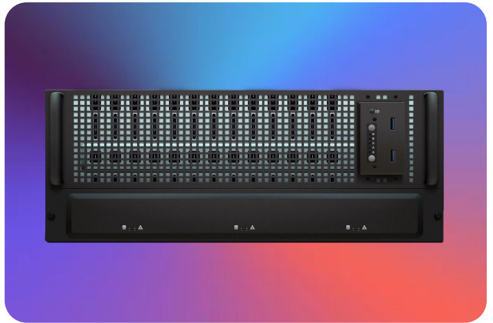
//TANK CHASSIS DIMENSIONS: 17" W x 37.4" D x 7" H
